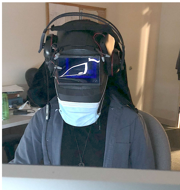
Figure 1. Viewing stimuli with the equiluminizing helmet. The screen display is reflected off the front blue filter. See Connolly, Connolly, Cleary, Herman, and Cavanagh (2017).
